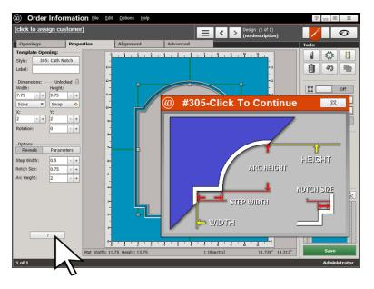
Note that the bright yellow lines and arrows in the **Parameter Map** also show exactly where the opening's size is measured.
